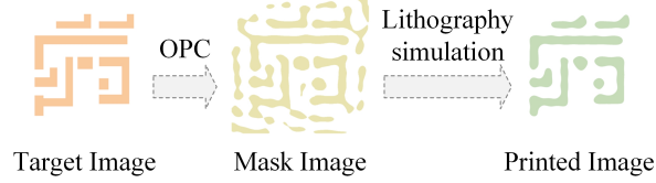
Figure 2. OPC and lithography simulation flow.
